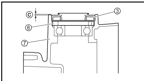
**INSTALLING THE BEARING AND OIL SEALS**
