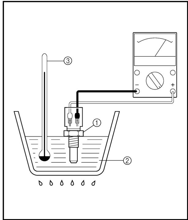
• Does the coolant temperature sensor operate properly?
