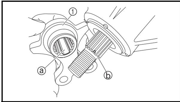
**INSTALLING THE PITMAN ARM**
