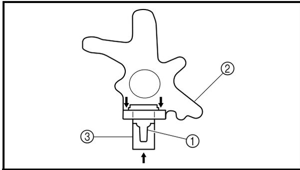
c. Remove the ball joint.
