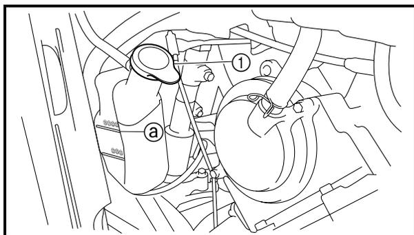
4. Remove the reservoir cap (1), add coolant or distilled water to the maximum level mark (a), install the reservoir cap, and then install the panel.
