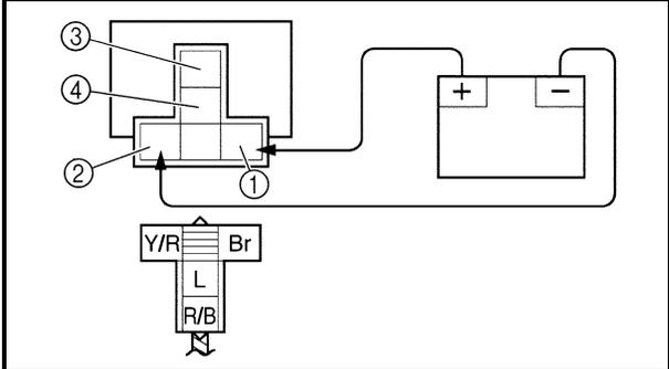
• Does the radiator fan motor relay have continuity between red/black and blue?
