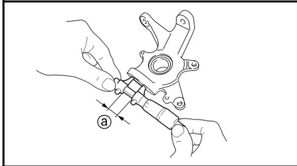
d. Measure the ball joint bore inside diameter (a).
