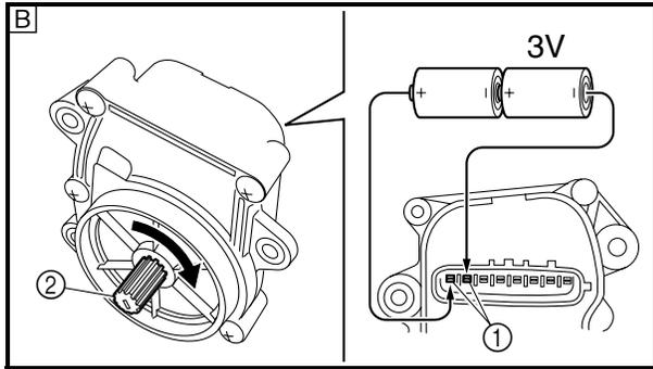
**B** Check that the pinion gear ② turns clockwise.
