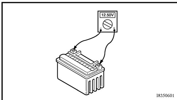
**Positive tester probe** → positive battery terminal
