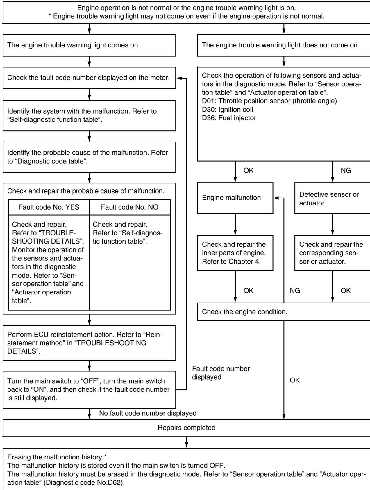
\* Operated when the engine trouble warning light is on.
