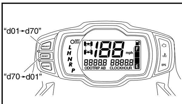
4. Simultaneously press the "SELECT" and "RESET" buttons for 2 seconds or more to execute the selection.
